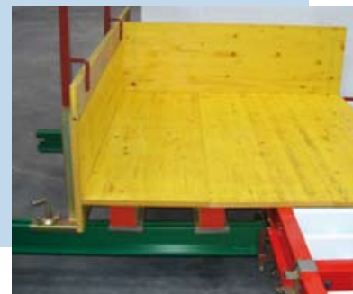
Compensation with beam and stop-end angle
